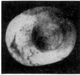
FIG. 1. Single crystal iron sphere with small flat after distortion by spinning.
